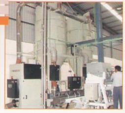
**FPL** added ZSK72 twin screw line with Brabender feeders and Conair dryer to double its capacity. This line is controlled with Allen Bradley software ensuring excellent consistency of product. **FPL** also underwent a total change in material handling system to improve its cost efficiency.
